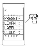
"LEARN" appears on the LCD display, and component names are displayed on the labels.
